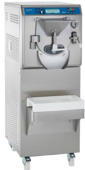
Any syrup or flavours that are required are introduced into the cylinder and mixed through with the agitator. During this phase, the machine incorporates air into the mix and begins to freeze as the base makes contact with the side of the cylinder, forming tiny crystals which give gelato its smooth characteristic.
