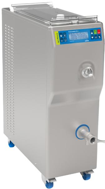
Pasteurisation is a heat treatment that ensures the safety of the ingredients and preservation of the gelato. After heating, the liquid mixture remains at an elevated temperature for the time necessary to guarantee the process; then cooled rapidly before being stored at a maximum of +4°C.
