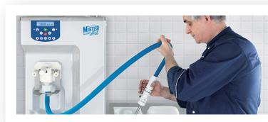
A hose and portioning piston is used to easily fill gelato cake and stick moulds.
